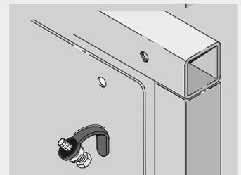
When the screw is released, it is still connected to the guard.
