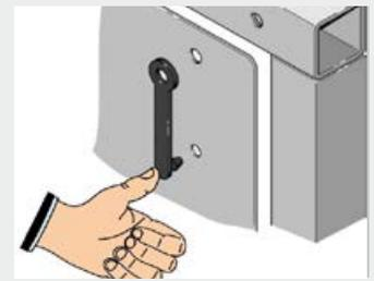
Press the mounting peg into the retaining hole.
