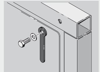
Push screw (with washer) through the holes in the ScrewClip and in the guard.
